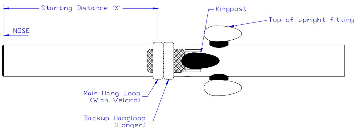
The hang loop is attached around the keel and should be within the following range. A recommended starting position is also shown. (If for example the hang loop had been removed and you are not sure where to replace it.) When you get the best position for your self, mark the keel with a felt tip pen or record a measurement for future reference. (See also Tuning p 13.)
