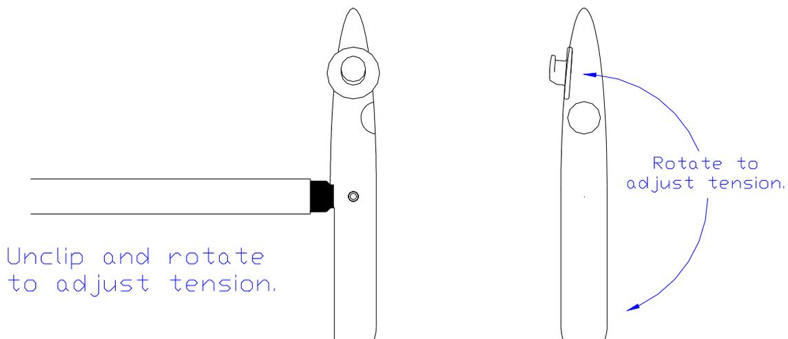
The Rio 2 battens are similar in design to those used in the high performance Cheetah and Evo competition gliders from Avian. The snap fitting allows neat robust fitting, easy rigging and easy precise adjustment of batten tension. The batten tension does make a difference to how the glider flies and is therefore important. The tension can be adjusted by rotating the clip end when open. One turn alters the tension by 1mm.
